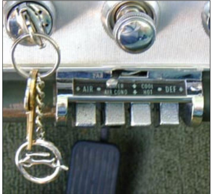
If you can live with the significantly higher cost of R-12 Freon®, you'll get much better cooling from the factory air conditioning on 1964 and older Impalas. If you do convert to 134a refrigerant, make sure you replace your condenser with one designed for 134a; it makes a big difference.
