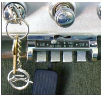
If you can live with the significantly higher cost of R-12 Freon®, you'll get much better cooling from the factory air conditioning on 1964 and older Impalas. If you do convert to 134a refrigerant, make sure you replace your condenser with one designed for 134a; it makes a big difference.
